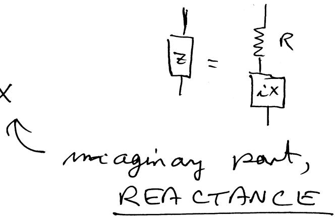
We will show it is only the real part of  $Z$  that leads to energy loss - the REACTANCE does not cause any energy loss
