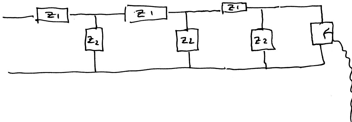
build a circuit element with an impedance  $\propto Z_0$  to mimic the rest of the ladder.
