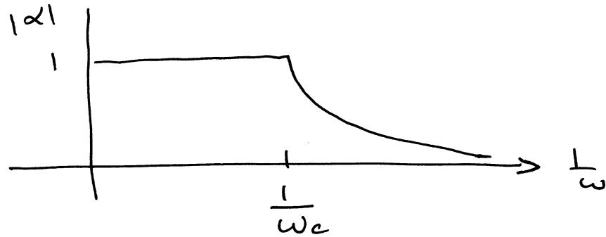
So for  $\frac{1}{\omega} < \frac{1}{\omega_c}$ , no blocking of signals
