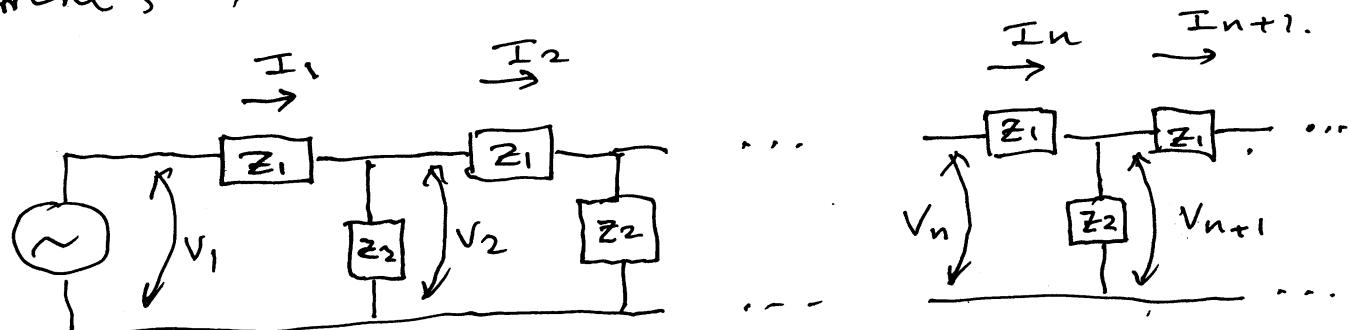
$$V_{n+1} = V_n - \underbrace{I_n Z_1}_{\text{voltage drop}}$$
