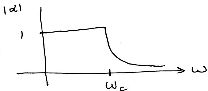
This is called a "low pass filter": signals with frequency  $\omega < \omega_c$  free pass through the ladder network, signals with  $\omega > \omega_c$  are rapidly attenuated and do not pass through the ladder network.
