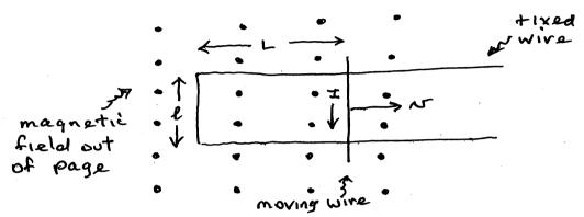
Lorentz force  $\vec{F} = q\vec{v} \times \vec{B}$  (there is no force due to the magnetic field on the charges in the stationary parts of the wire). In the case of the geometry shown, this force is of magnitude qvB and points downwards, and so will set up a current I in the direction shown. Recalling that the EMF is the work per unit charge done by the force, and that the force actions only in the moving portion of the wire,
